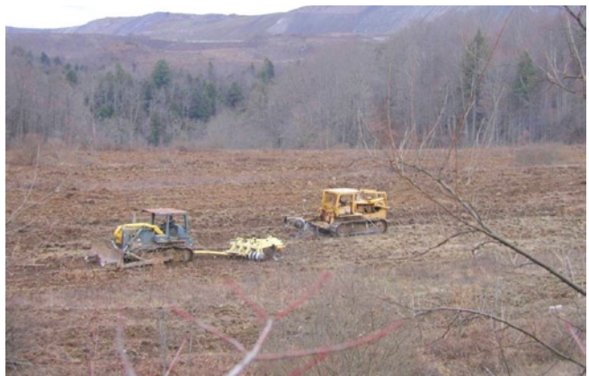
Figure 9. Preparing an area for reforestation research at Powell River Project Research and Education Center. The large disk (left) is used first to break up the sod, then an advanced deep-tillage device (right), was used to prepare the land for planting.
