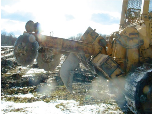
Figure 6. An example of a soil ripping tool (Savannah-type plow) used to prepare several mine sites in Wise County, Virginia, for reforestation in late 2007. The ripping shank is 36" long and the large steel wheels on the end of the shaft behind the ripping shank ("coulters") are 30 inches in diameter. The coulters are intended to push a mound onto the top of the ripped channel, where trees can be planted.
