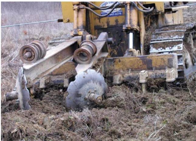
Figure 7. An advanced tillage tool intended for use on mined lands. A center shank (not visible) rips a deep trench through the compacted mine soil while the coulters produce a mound of loose soil over the rip where the trees are planted. Smaller shanks (up to six) to the right and left break up the surface on either side of the planting location to a depth of 12-to-18 inches; the top of one such smaller shank is visible as it enters the soil on the right hand side of the tool bar.
